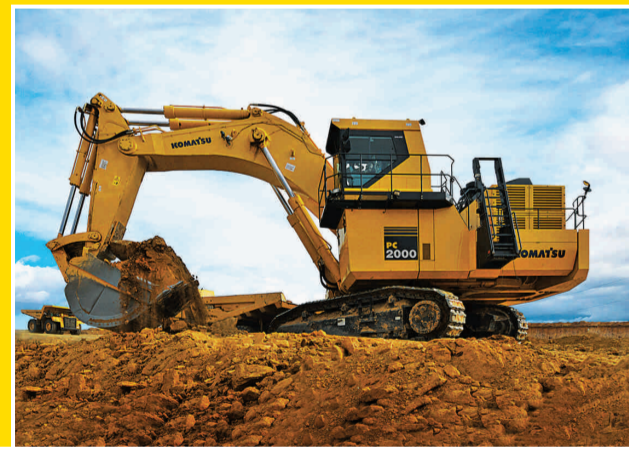
Hydraulic Excavators Backhoe
