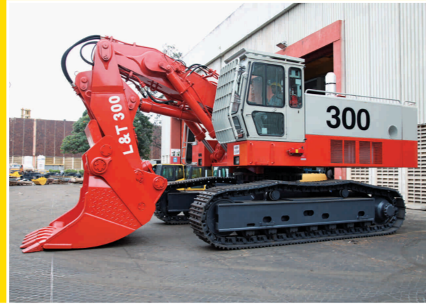
L&T 300 Hydraulic Excavator
