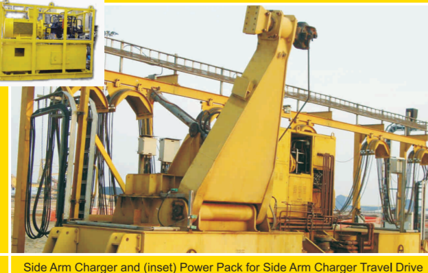
Side Arm Charger and (inset) Power Pack for Side Arm Charger Travel Drive
