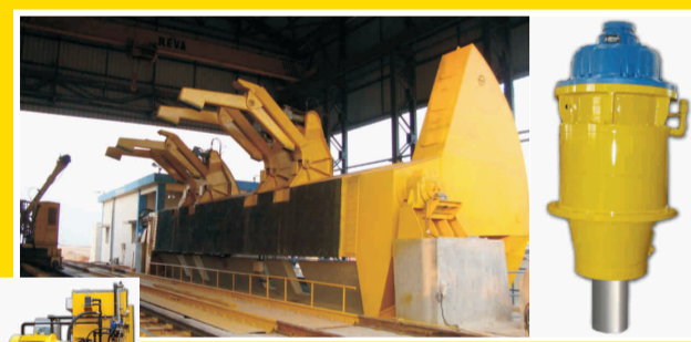
Wagon Tippler and (inset) Power Pack for Wagon Clamp & Tippler Drive Hydraulic Drive
