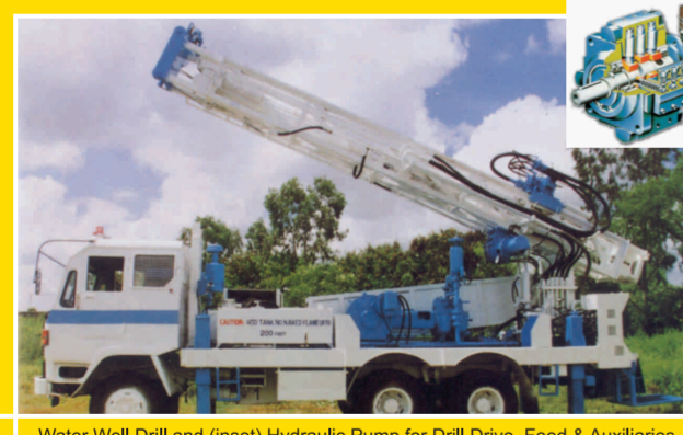
Water Well Drill and (inset) Hydraulic Pump for Drill Drive, Feed & Auxiliaries
